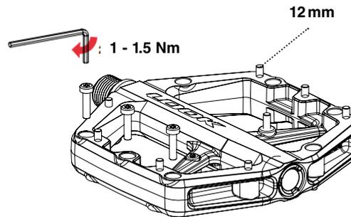
**Warning:** If you need to remove or install the pins, use a T10 Torx wrench and observe a tightening torque between 1 and 1.5Nm maximum. Before tightening / loosening, ensure the pin heads are clean.
