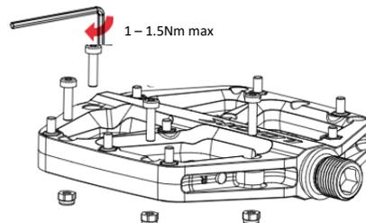
**Warning:** If you need to remove or install the pins, use a T10 Torx wrench and observe a maximum tightening torque of 1 – 1.5 Nm. Before tightening / loosening, ensure the pin heads are clean.
