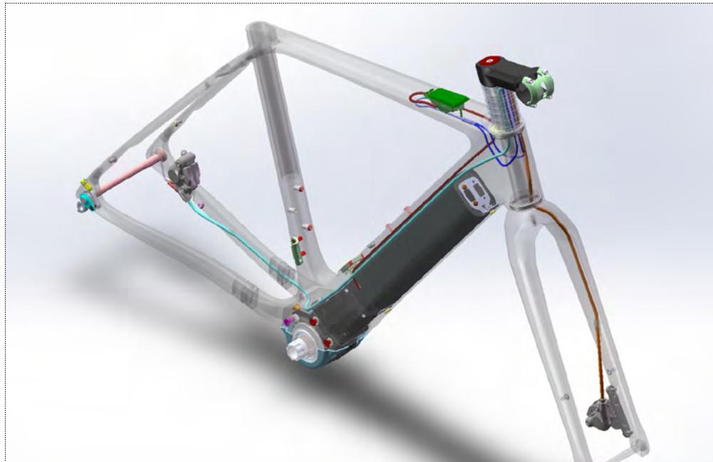
**1** - To assemble the frame, it is preferable to hold it by the seat post at a torque of 7 Nm. Initially, the frame should be bare to facilitate access through the headset and bottom bracket, allowing you to place the rear disc brake hose. Use foam tubes of 510 mm length for each brake hose to limit noise in the down tube.
