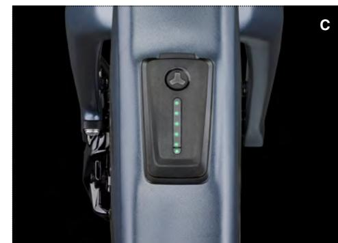
If the LED HUB is off, the bike is powered off OR the LED HUB is faulty.
