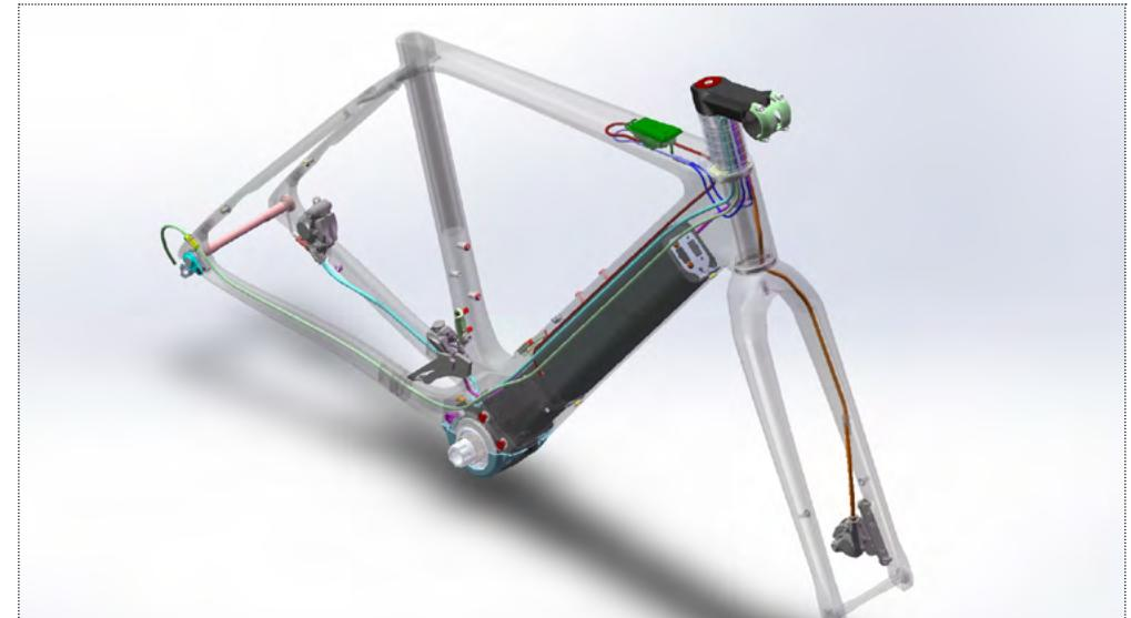
**1** - To assemble the frame, it is best to hold it by the seat post at a torque of 7 Nm. Initially, the frame should be bare to facilitate access through the headset and bottom bracket, allowing you to place the cables in the down tube and then the guide (Fig. 1) to the front and rear derailleurs and the rear disc brake. Use foam tubes of 510 mm length for each cable and brake hose to limit noise in the down tube.
