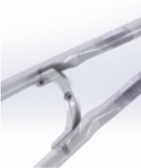
Secure the fender to the frame at the back of the bottom bracket using the  $\text{Ø}12$  spacer, length 15, and the CHC M5x30 screw.
