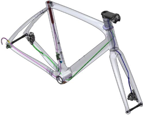
**1** - You will need a workshop stand to assemble the bike. It is important to secure the frame by the seatpost, tightening to a torque of 7Nm. The frame must be stripped to allow easy access to the headset and bottom bracket, allowing you to route the brake hoses and e-tubes according to SHIMANO's instructions, from the battery in the seat tube to the front and rear derailleurs. Use 510mm-long foam tube on the rear brake hose to eliminate any unwelcome noise in the downtube.
