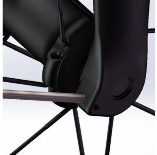
Fit the stays to the fender using the base lock nut on the outside and the TBHC M4x8 screw and washer on the inside of the fender.
