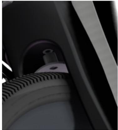
Secure the fender to the rear of the seat tube using the CHX M5x20 screw.
